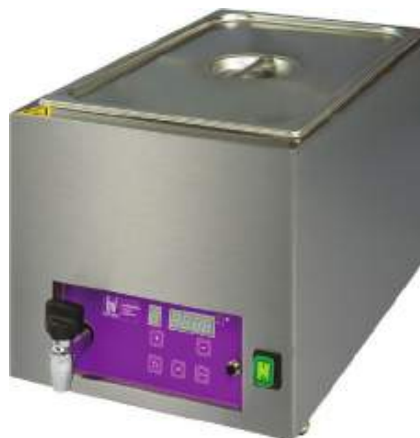
STATICOOK Stainless steel (AISI 304) body, digital panel with 10 programs, timer, internal memory, practical basket with removable dividers, core probe and delayed start. Cooking time 0-48h
