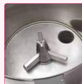
Residual water drain
